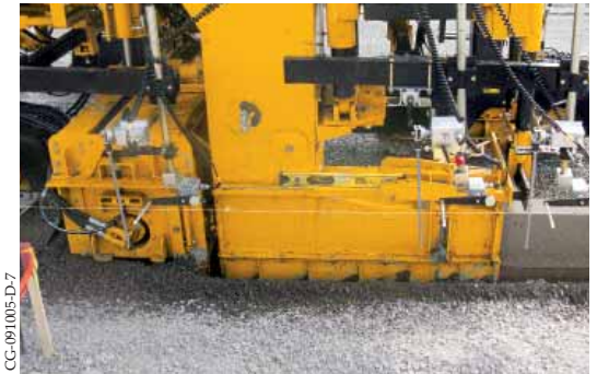
The steer sensors automatically adjust trajectory in and out of tight radii as the GT-3600 moves forward.
